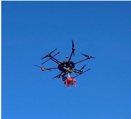
people and property. The RDS1's one-of-a-kind controlled freefall delivery technique also enabled pilots to reduce time on-site to under 30 seconds per delivery. Shaving seconds from each delivery allowed DroneUp to extend the range of its flight platform and service a greater geographic area around each delivery hub while reducing the safety risk and noise pollution to residents.
